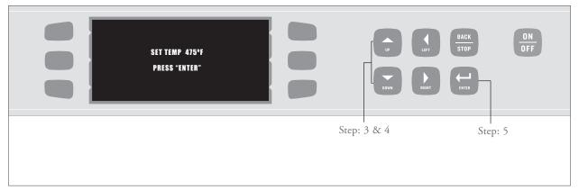
FIGURE 14: Adjusting the Cook Chamber Temperature
